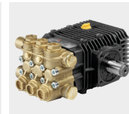
Triplex pump, ceramic pistons and brass head
